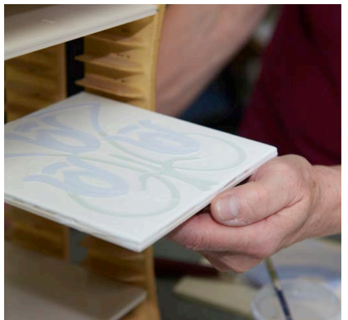
4. When all the colours have been applied, the tile is inspected, loaded into a crank and then left to dry, before being fired in the kiln.
