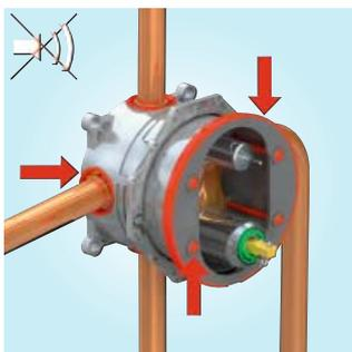
**Soundproof.** The brass body of the iBox universal rests on seals to prevent the noise from water passing through the wall. The screwed joint is between the collar and housing of the iBox universal, but not the function block, which prevents sound from travelling through to the tile.
