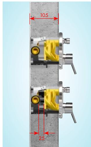
**Basic set extension.** Hansgrohe has a solution, even for a situation where the iBox universal has been fitted too deep into the wall. Then the basic unit extension is fitted between the connector and the function block. The extension set ensures safety right up to the wall, in this case preventing damp walls.
