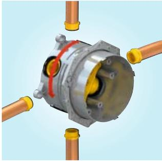
**Installation with rotational symmetry.** The symmetrical construction of the iBox universal makes all connections simple. It is important that the cold water is on the right simple the hot water is connected opposite to it. When using a shower mixer the top or bottom connection point can be used.
