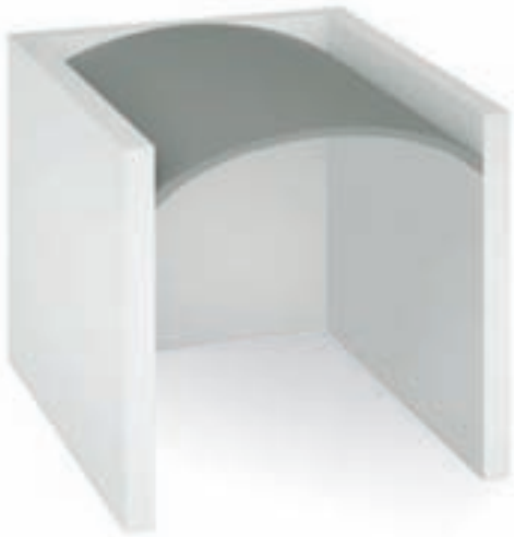
Volta a botte Barrel vaulted ceiling
