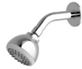
37150-000/1C-I011 Wall-mounted shower set Faceplate: 3 inch External thread: G1/2B OD of flange cover: Φ 60mm Brass alloy shower arm Chrome finish ABS raincan
