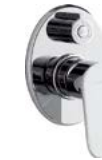
37130-239/1B3-1 Concealed diverter (two-way) External thread: G1/2 OD of flange cover: φ150mm Solid brass Φ40 ceramic cartridge Chrome finish Match with model:37155
