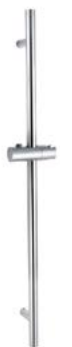
T5701-2B01-I021 Slide bar Installing distance: 750mm Total length: 900mm φ25 stainless steel tube Adjustable hand shower bracket
