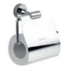
935007-1D-I011 Tissue holder 150x68x140mm Brass alloy base Zinc alloy body Stainless steel cover Chrome finish
